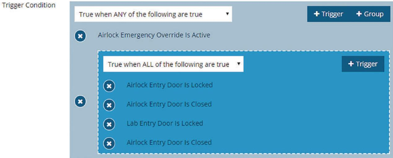
If the emergency override input is active, then the *Airlock Access Allowed* custom output will always be on, ignoring the states of the doors. This lets all of the other logic using this custom output to remain unchanged.
